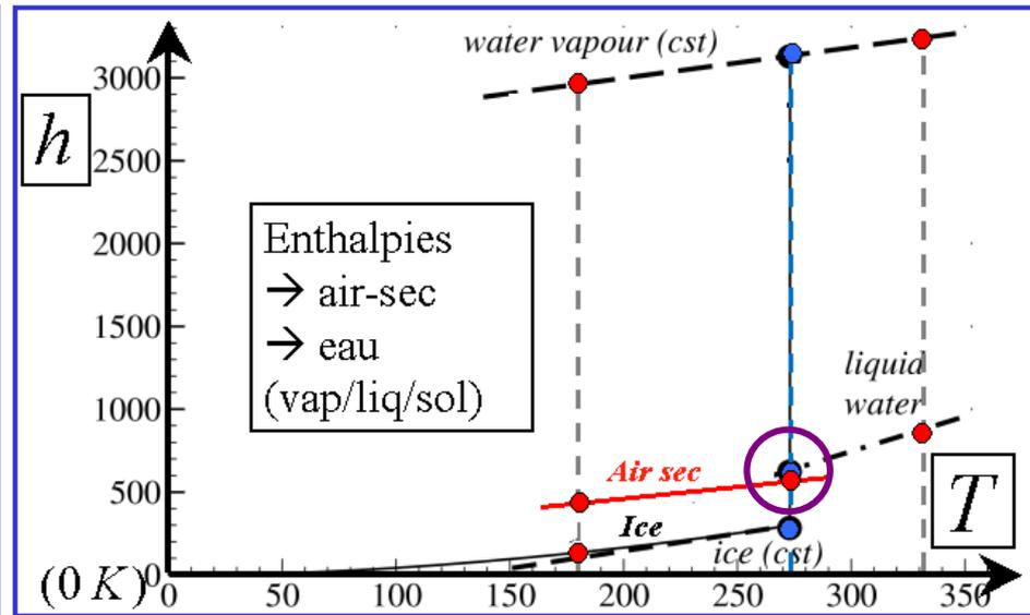
*Enthalpy diagrams (in kJ/kg) for  $N_2$ ,  $O_2$ ,  $H_2O$  and for a 1000 hPa pressure*
