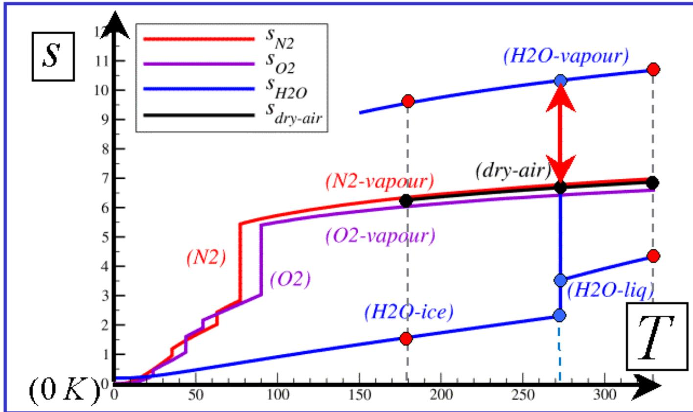
*Entropy diagram (in kJ/K/kg) for  $N_2$ ,  $O_2$ ,  $H_2O$  and for a 1000 hPa pressure*
