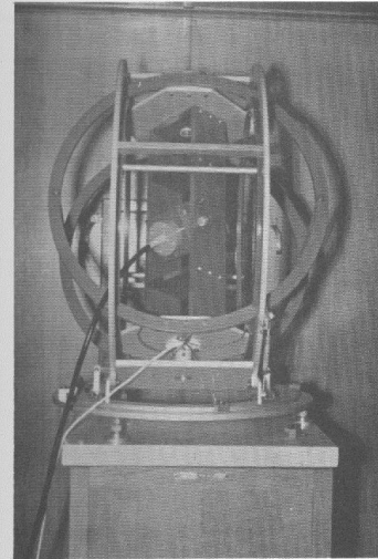
Figure 2 Helmholtz Coil System
